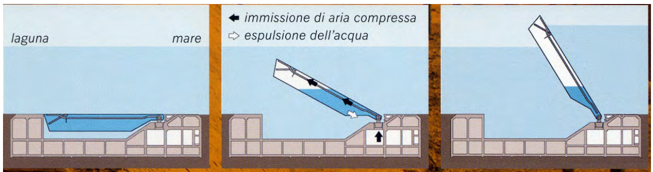
5. Mechanism of operation of MO.S.E.
